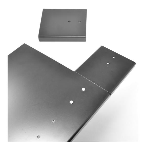
**STEP 3:** Use the rightmost two holes on the extender bracket to line up with the two rightmost holes in the G1000 Avionics Panel as shown below and use the remaining M4x12mm screws, washers, and nuts to secure the avionics panel to the avionics table uniformly along the front lip. Use the universal wrench to prevent the nuts from turning while tightening.
