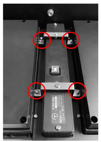
WARNING: DO NOT OVERTIGHTEN AND DO NOT SUBSTITUTE LONGER SCREWS THAN PROVIDED BY REAL SIM GEAR OR THE SCREWS MAY PENETRATE THROUGH THE FACE OF THE G1000 HOUSING! **STEP 2:** Detach all avionics/accessories from the Volair Sim avionics table except for the yoke (if installed). If you do not have the yoke installed, test-fit it now. Volair Sim Avionics Panel G1000 is compatible with the following flight yokes: Logitech (Saitek), Honeycomb Alpha, Yoko, and Brunner.
