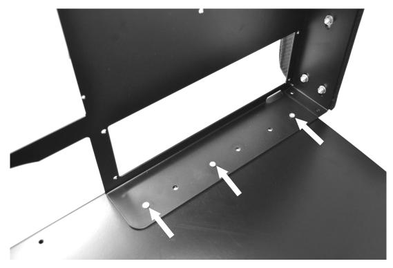
**STEP 4:** Attach the two (2) rear support brackets as shown below by loosening two (2) nuts underneath the Avionics Panel glare-shield. Ensure that the position of the brackets will not interfere with the Yoke/Throttle panel installation. Gently push the front of the Avionics Panel towards the back to slightly pre-load the support brackets. When satisfied with the position, tighten the nuts under the glare shield.
