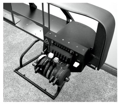
NOTE: IT MAY BE HELPFUL TO TEMPORARILY REMOVE THE MFD OR LOOSEN THE MOUNTING SCREWS OF THE AVIONICS PANEL DURING THE INSTALLATION.
